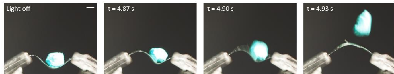
Figure 1: Snap-through of LCN. Snapper is 1 mg, ball is 2 mg and scale bar corresponds to 2 mm.
